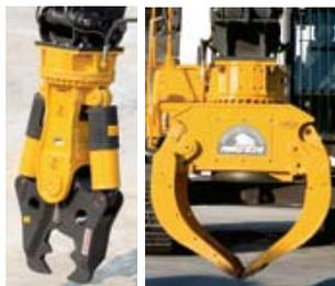
Volvo hydraulics are ready for a range of demolition **attachments** including **grapples, hammers, shears** and **pulverizers**.
