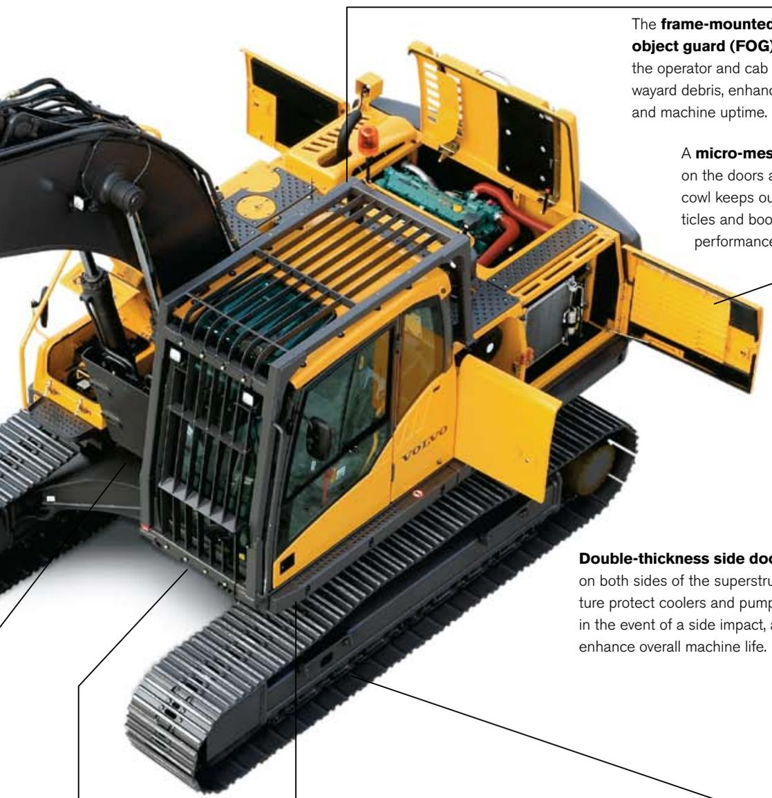
The **frame-mounted falling object guard (FOG)** protects the operator and cab from wayard debris, enhancing safety and machine uptime.
