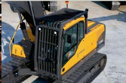
• Frame-mounted FOG protects the operator.
