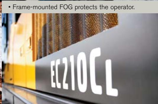
• Micro mesh screens keep particles from coolers.
