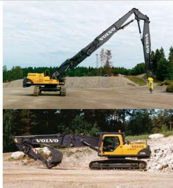
• Easily change from demolition configuration to straight boom or regular backhoe.
