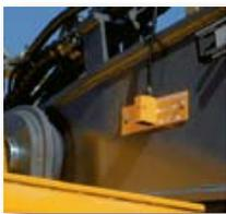
Boom-mounted **Total Moment Indicator** provides warning if the HR excavator is approaching maximum safe load.
