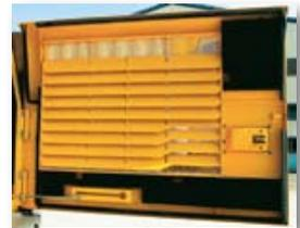
The bolt-on **side impact protection system** protects the superstructure from damage.
