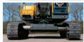
**Full-length track-chain guards** keeps out demolition debris and prevents rebar or other sharp objects from lodging in the tracks. Extendable undercarriage expands by 1 m (3' 3") for increased stability.
