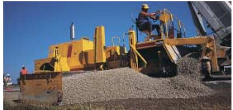
The conveyor will discharge material from either side of the machine. Discharge direction, left or right, is controlled with an electrical switch on the operator's console. Note that to accommodate opposite side discharge, it is necessary to transfer the strike-off assembly, hopper confining chutes, operator's console and seat to the opposite side of the machine. Unless otherwise specified, all RW-195D Road Wideners are shipped from the factory set-up for right side discharge.
