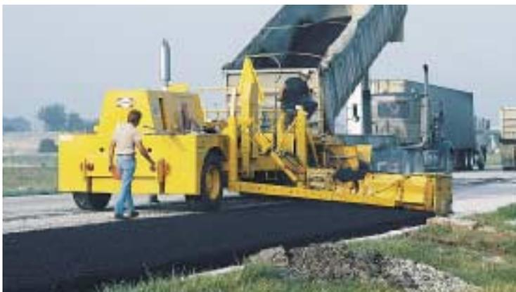
**Suspension:** 385/65R22.5 radial pneumatic tires, hydroflated to provide maximum tractive effort, then inflated to 105 psi (725 kPa).
