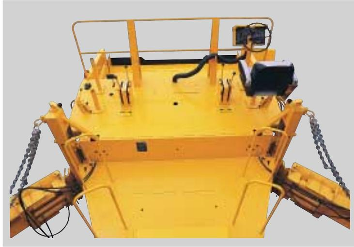
Control functions located on the operator's console include main power, starter throttle, horn, conveyor speed, shuttle and discharge direction, strike-off lift and lateral movement, hopper lip position and front and rear steering.
