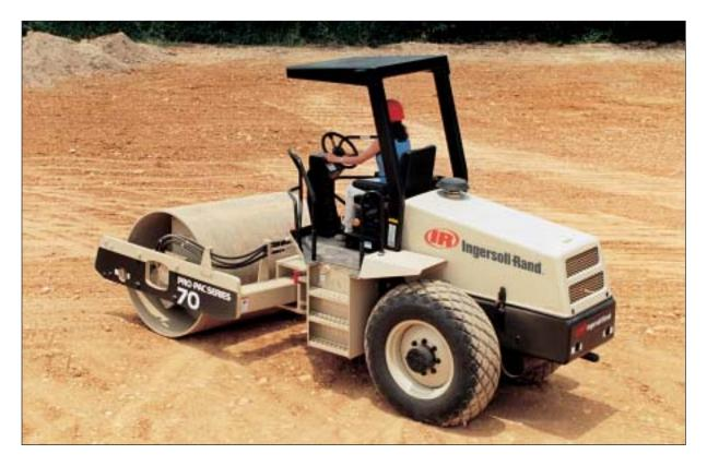
The Ingersoll-Rand SD-70 PRO-PAC<sup>™</sup> Series features a Cummins turbocharged 4-cylinder diesel engine. The 95 hp (71 kW) liquid-cooled engine provides greater power and torque to handle the increased demands of projects at higher elevations, improved gradeability and propulsion through highly cohesive soils. The lightweight, single-piece engine enclosure is hinged at the rear to allow unobstructed access to the engine, radiator, battery, filters and daily maintenance check points.
