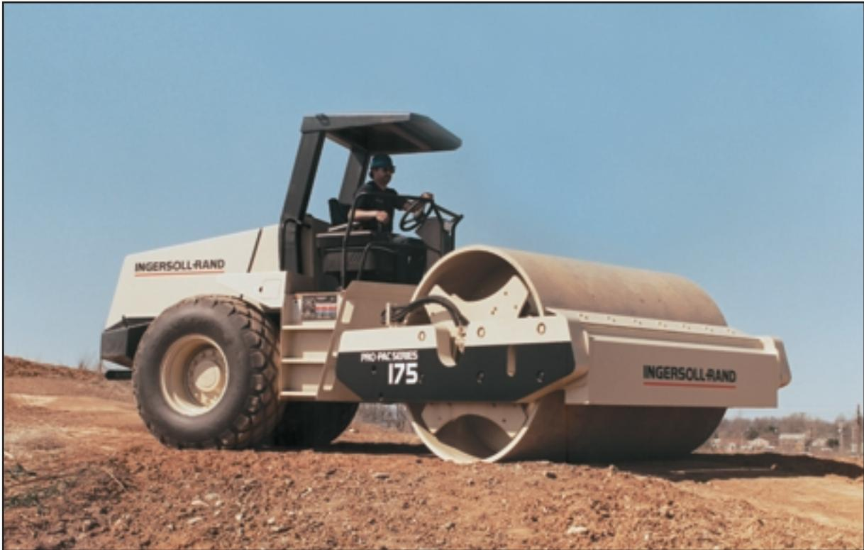
The Ingersoll-Rand SD-175 PRO-PAC Series features a powerful Cummins turbocharged and aftercooled C8.3-C diesel engine. The 205 hp (153 kW) liquid-cooled engine and heavy-duty hydrostatic transmission provides power and torque to handle the demands of projects at elevations, in cohesive soils and climbing steep slopes. The lightweight, single-piece engine enclosure is hinged to allow unobstructed access to the engine, radiator, battery, filters and daily maintenance checkpoints.
