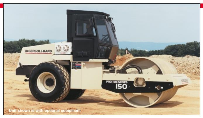
The Ingersoll-Rand SD-150 PRO-PAC Series features a powerful Cummins turbocharged and aftercooled B5.9 diesel engine. The 185 hp (138 kW) liquid-cooled engine provides greater power and torque to handle the increased demands of projects at higher elevations, operation on steeper slopes and propulsion through highly cohesive soils. The lightweight, single-piece engine enclosure is top hinged to allow unobstructed access to the engine, radiator, battery, filters and daily maintenance checkpoints.
