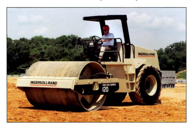
The Ingersoll-Rand SD-120 PRO-PAC features a powerful Cummins B5.9-C diesel engine. This six-cylinder engine provides power and torque to handle the increased demands on projects like high altitude operation and compaction of highly cohesive soils.
