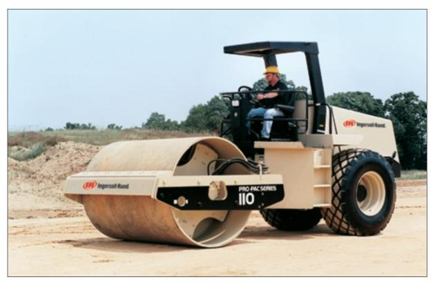
The Ingersoll-Rand SD-110 PRO-PAC Series features a powerful Cummins B5.9-C engine. This six-cylinder engine provides greater power and torque to handle the increased demands on projects like altitude operation and compaction of highly cohesive soils.
