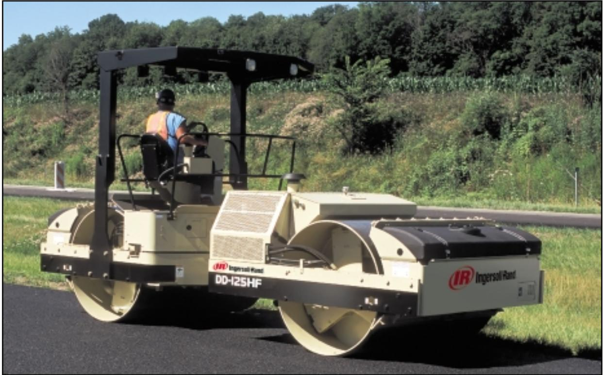
The DD-125HF features dual 84 inch (2135 mm) wide drums with 3200 vpm (53.3 Hz) frequency for high performance capability on main line highway and other large paving jobs. Operating weight of 14 tons (12.7 metric tonnes) meets all state D.O.T. static rolling requirements. The DD-125HF has a nominal capacity to more than 385 tons (240 metric tonnes) of HMA per hour.
