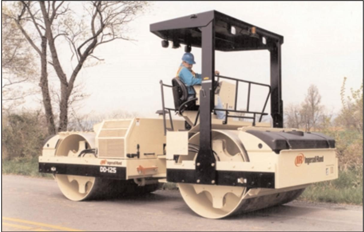
The DD-125 features dual 84 inch (2135 mm) wide drums with 2500 vpm (41.7 Hz) frequency for high performance capability on main line highway and other large paving jobs. Operating weight of 14 tons (12.7 metric tonnes) meets all state D.O.T. static rolling requirements. The DD-125 has a nominal capacity to more than 300 tons (265 metric tonnes) of HMA per hour.
