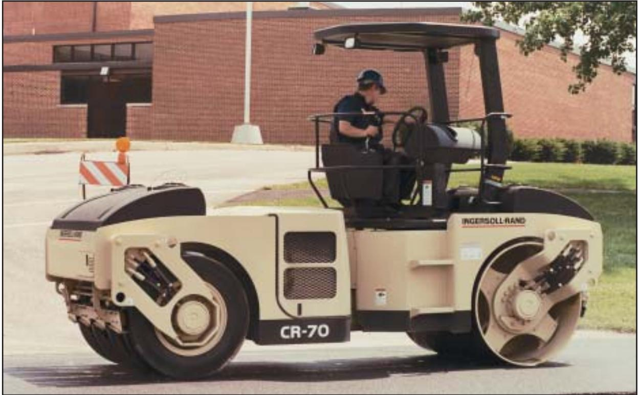
The CR-70 is a 6.5 ton (6 tonnes) weight unit that utilizes the forces of vibration and tire manipulation to achieve required density and smoothness on Hot Mix Asphalt (HMA) pavements. The unit can also be used to compact granular or mixed soils, crushed aggregates and cement-treated bases.
