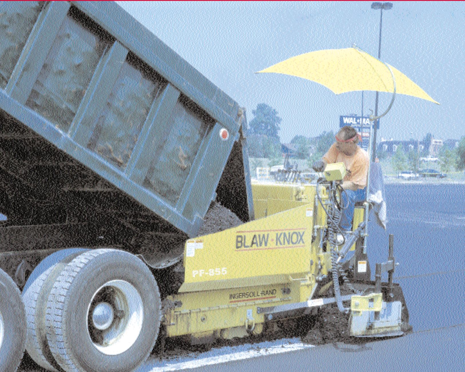
The **PF-855** is a track mounted paver/finisher with standard paving widths of 8 to 12 ft. The material delivery system is a 7 ton capacity automatic dual conveyor system. The PF-855 is designed for high efficiency on large commercial jobs. Typical applications include secondary roads, commercial parking lots and drives.
