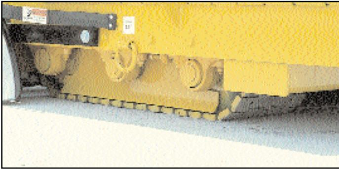
**Steering:** Cable-free hydraulically actuated steering via 4 separate counter rotation valves w/ neutral safety lock.
