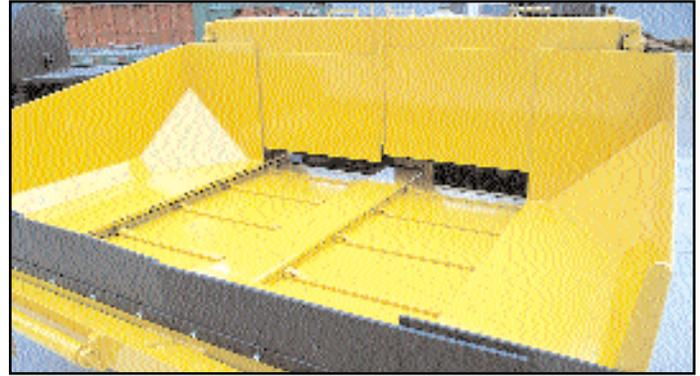
**Paving Depth:** 0-6" / manually adjustable with two bearing-free depth adjustment jacks. Depth indicators are standard.
