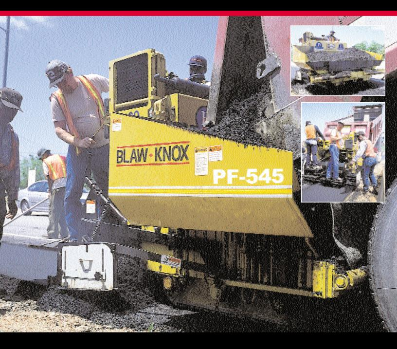
The **PF-545** is a unique track mounted paver/finisher with standard paving widths of 5 to 8 ft. The material delivery system is a 4 ton capacity automatic dual conveyor system. The PF-545 is designed specifically for paving in restricted sized areas. Typical applications include cart paths, recreational trails, trenching and road widening.
