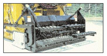
**Augers:** Two independently operated 8" augers w/ forward and reverse / mounted on extensions. This gives you the ability to retract extension and auger material to the main screed without bending end gate.
