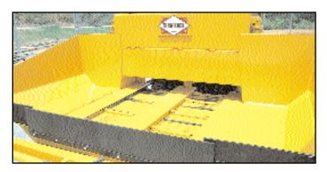
Material Delivery: Two 18" wide independently operated conveyors w/ automatic or manual operation for conveyors and augers. System is triggered by two electronic sensors mounted on the extensions.
