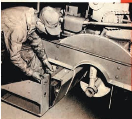
• Bottom: Operator placing narrow Screed Extension in place for bolting. One section of tamper is in place and Auger Extension Socket is shown.
