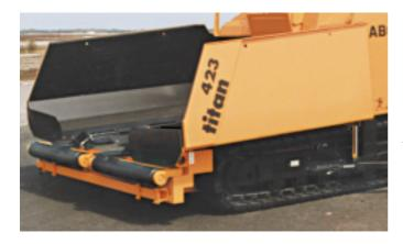
Hydrostatic individual drives for each conveyor and each distributing auger:
