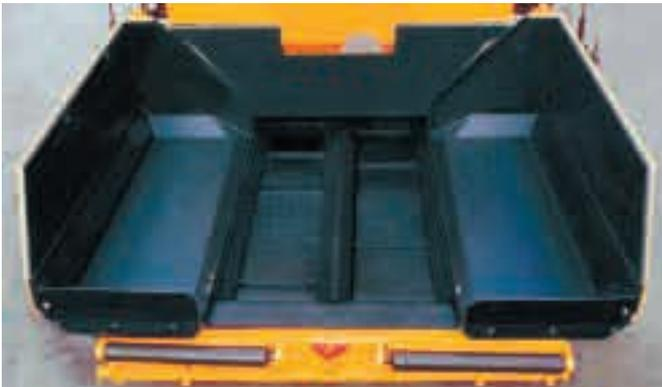
Individual hydrostatic drives for each conveyor and each distributor auger:
