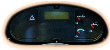
The nerve center of the "B" Series operator environment is the Contronic Monitoring System. This multi-function system tells the operator the status of all machine functions, including engine RPM, engine temperature, fuel level, ground speed, filter restriction, differential lock/unlock and many others. Contronics tells the operator what is happening with the machine as he or she operates it.
