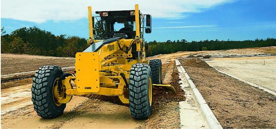
Whatever your application, the Volvo All Wheel Drive System is tuned to the task. The system provides an even distribution of power through independent variable displacement pumps and high torque motors at each front wheel. If the traction differs on either side, this system ensures that optimum pulling power is still achieved.
