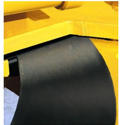
Duramide™ bearing material eliminates metal-to-metal contact and reduces the need for circle turn lubrication and adjustment. As well as being simple and cost-effective to replace, it has a minimum service life of more than 5,000 hours.
