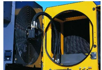
Since the grader's need for cooling depends on ambient conditions as well as the engine's power output, the variable-speed hydraulically driven fan on Volvo graders is designed to respond to actual demand. Combined with non-stacked coolers, the system continuously delivers just the right amount of cooling effort, consuming less fuel, producing less noise and maximizing available power for other grader functions.
