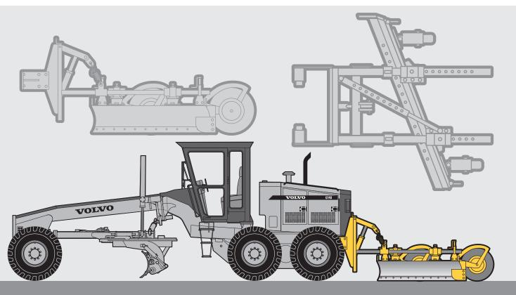
The Volvo Windrow Eliminator is used for one pass road surface or road shoulder maintenance. The Windrow Eliminator mounts to the rear of the grader and re-distributes the windrow from the grader moldboard eliminating a second pass, saving time and increasing efficiency.
