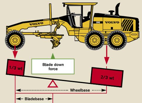
$$\text{Blade down force} = \frac{\text{front weight} \times \text{wheelbase}}{\text{wheelbase} - \text{bladebase}}$$
