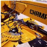
Patented dual-cylinder circle drive uses direct-acting hydraulics for exceptional turning and holding power under full load. DURAMIDE faced clamp plates and guide shoes prevent metal-to-metal contact; and provide longer service life and less maintenance than metallic systems.
