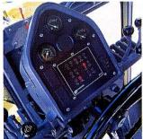
Pedestal includes a 3-level electronic monitor to alert operator to machine status, with backlit switches and fuel level, engine oil pressure and engine coolant temperature gauges.
