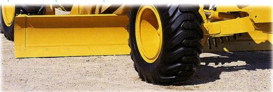
With its 72° front axle steering arc, Series IV moves comfortably in confined work areas. The tight turning radius means faster finishing in cul-de-sacs and less following-up in the corners.
