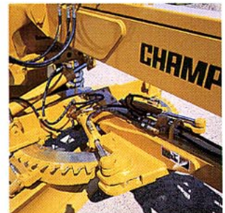
Patented dual-cylinder circle drive uses direct-acting hydraulics for exceptional turning and holding power under full load. DURAMIDE faced clamp plates and guide shoes prevent metal-to-metal contact; and provide longer service life and less maintenance than metallic systems.
