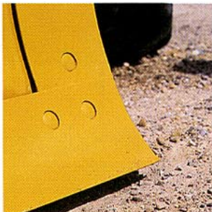
Boron steel cutting edges with 6" bolt spacing. Top and bottom slide rails are supported on DURAMIDE™ bearings, minimizing free play for fine grade control.
