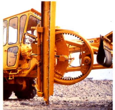
Safety clutch for the swinging function of the grader blade.
