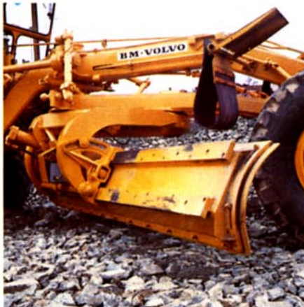
The wear parts of the grader blade are readily replaceable. The illustration shows the version of the grader blade with hydraulic setting of the blade pitch (optional extra).
