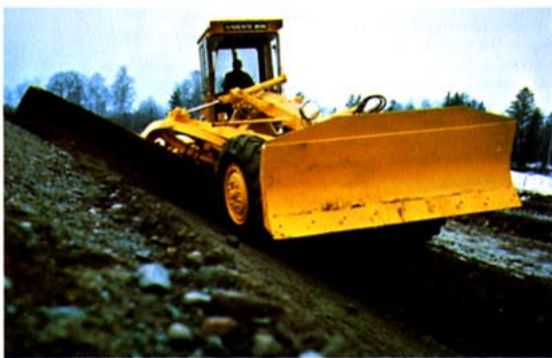
Individual adjustment of the rotation circle and blade give the 3500 very wide reach to both sides.
