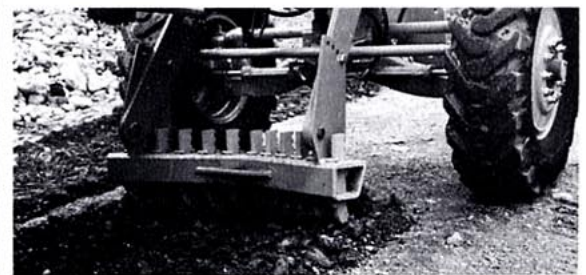
2. Above. Hydraulically operated front blade. 3. Below. V-type scarifier, mounted in front of the mould-board.
