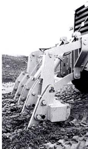
1. Rear mounted ripper. Standard arrangement includes 5 heavy-duty shanks.
