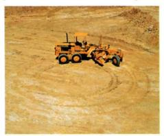
With a turning radius of only 7.5 metres (25 ft), the 3300 is highly manoeuvrable. Sharp bends can be taken with a full load while the machine is steered with the bogie only.
