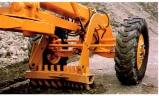
This attachment is mounted in front of the grader blade and is operated hydraulically. On the 3200, an extra hydraulic function must be installed for this attachment if the reserve function is already being used. Stable construction with ripper of Bofors steel. Working width 1 235 mm (4 ft), max. working depth 340 mm (1 ft 1 in). Weight 570 kg (1 256 lb).
