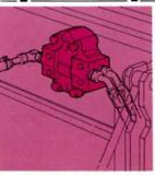
A powerful twin gear pump gives the dualcircuit system plenty of muscle.
