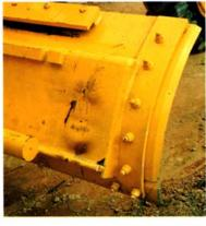
The rear side of the grader blade is of a completely new design with box welded reinforcement.
