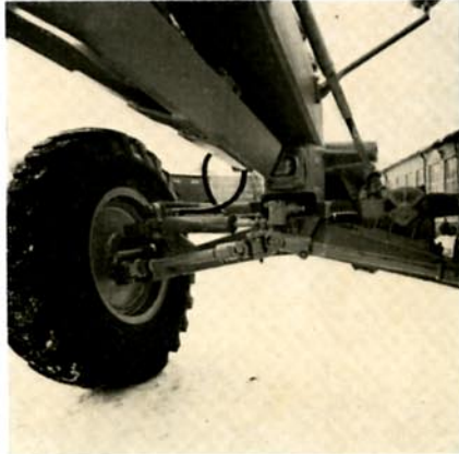
Hydraulic-assisted steering retains mechanical "feel". The mechanical steering system works independently of the hydraulic servo system.
