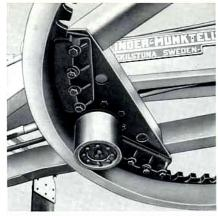
The adjustable blade circle guides, the teeth of the gear ring and the worm of the worm gear are subjected to special heat treatment. A safety clutch disengages the gear ring when running into solid obstacles.
