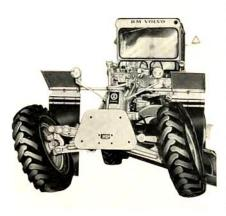
All universal joints for wheel inclination and steering have crosses journalled in needle roller bearings.
