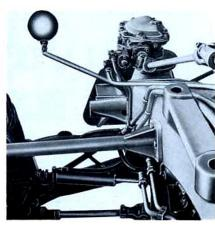
Hydraulic power-assisted steering with "mechanical feel". The mechanical steering functions independently of the power steering.
