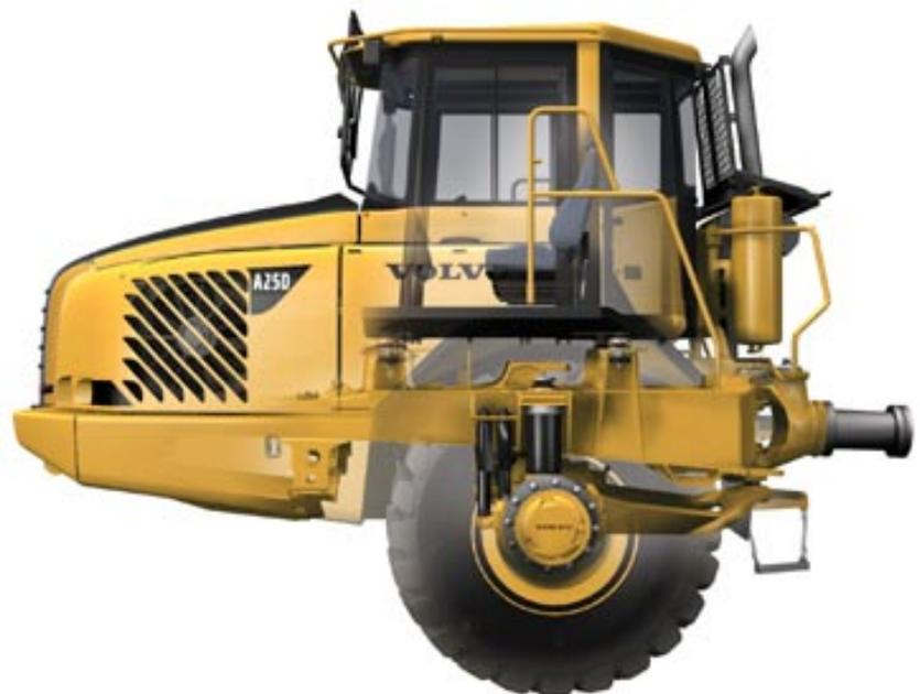
The reliable three-point suspension consists of heavy duty components. A durable design that gives a comfortable smooth ride.
