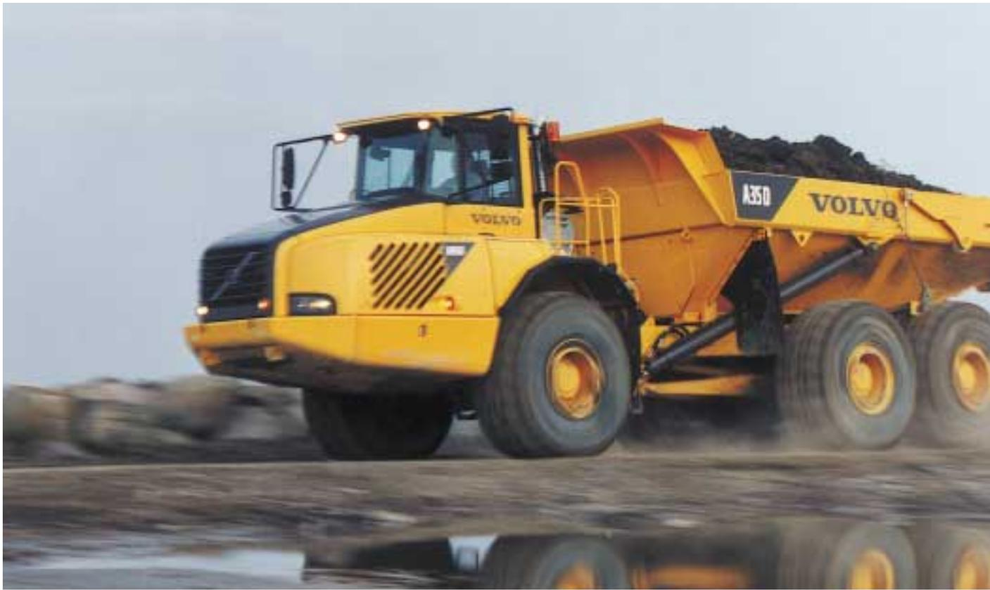
The front axle's sturdy rubber suspension with shock absorbers means the hauler can maintain high average speeds while maintaining operator comfort and minimizing mechanical wear. The bogie design means that each pair of wheels can move independently to maintain ground contact. This lets the body stay practically level over rough ground while the frame undergoes less stress.
