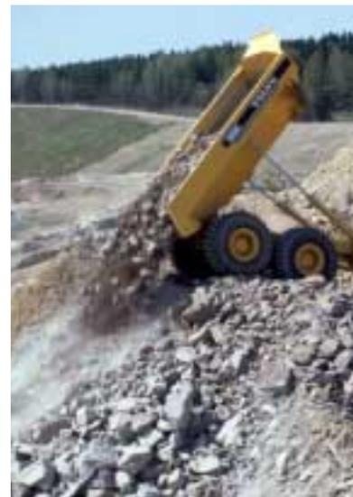
the body protects the cab and the operator, a wire-operated tailgate reduces the risk of spillage during haulage. Heating of the bottom of the body greatly reduces the risk that the load will stick under certain operating conditions. The exhaust gases are used for body heating, which means no extra energy is consumed.
