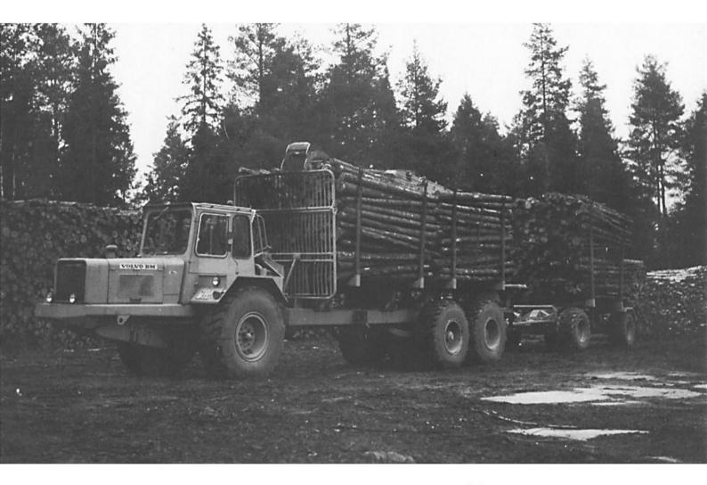
VOLVO BM 860 TC shortwood hauler for road hauling. Built with rear-mounted loader and trailer. Carries three stacks of 3-m pulpwood or logs.
