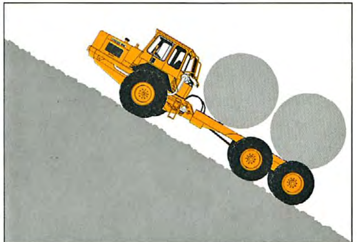
The 860 TC has excellent hill-climbing capabilities owing to its powerful engine, torque converter, 4-wheel drive and good weight distribution. At a total weight of 30 tons, the 860 TC can climb slopes of up to 30° at a coefficient of friction of 0.6 or higher.
