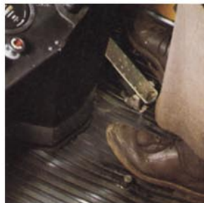
Foot switches enable differential locks to be easily engaged/disengaged.
