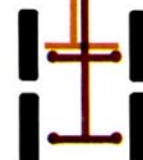
Safe brake system acting on all wheels.
