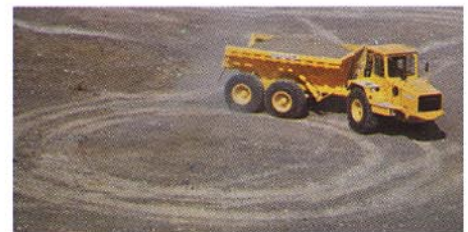
Articulated steering gives the 860 a small turning radius.
