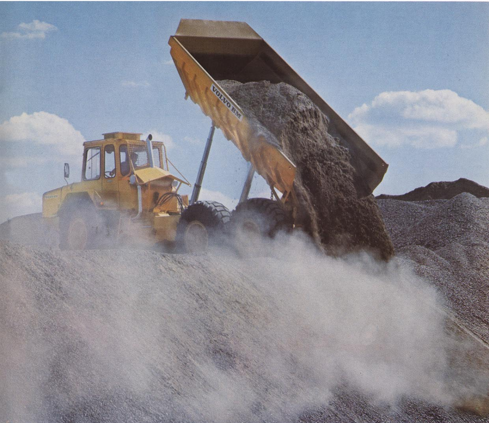
Rapid dumping thanks to a high angle – 70° – and an efficient hydraulic hoist system
