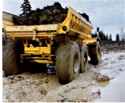
The 4-wheel drive and the differential locks can be engaged and disengaged while the machine is in motion to prevent loss of speed in tricky sections.
