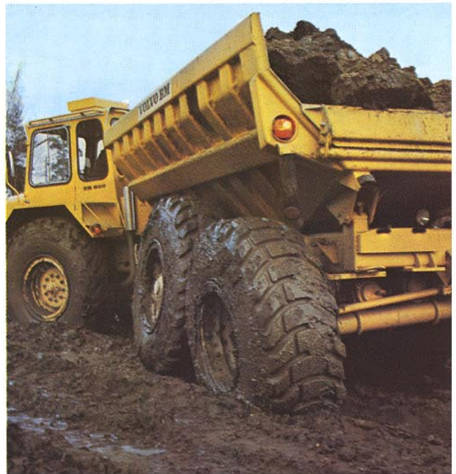
Minimum spillage as the body "floats" over the terrainequalizing bogie.
