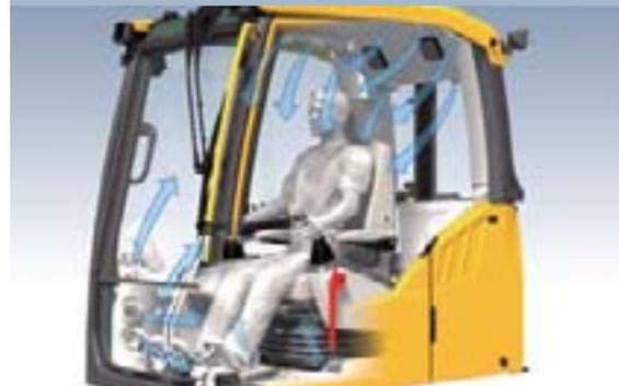
• Industry's highest heating/cooling capacity with 14 vents.
