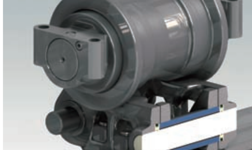
• Greased and sealed track link.
