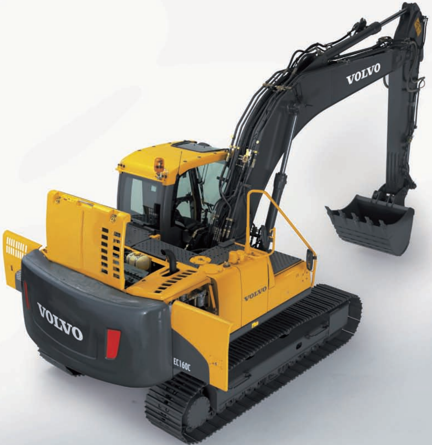
• Simplified, ground level service access.
