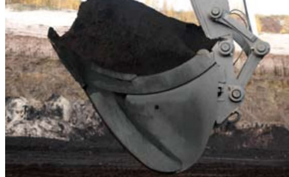
• General purpose (GP) buckets have rugged design and self-sharpening GPE teeth.
