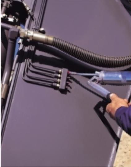
Exceptional ease in service and maintenance is seen in every detail of the Volvo excavator. It is designed for operator convenience and most maintenance can be done at ground level or from the service platform. Grease points are conveniently located and grouped together for easy service.
