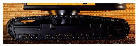
If you have to allow for transport restrictions, you should choose the narrower track undercarriage (2.49 m wide and prepared for dozer blade). The wider version is even more stable with higher lift capacity.
