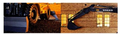
Articulated outriggers with lock cleat increase stability and reduce stresses on the ground. Good ground clearance, limited-slip differential and a design that permits the front axle to oscillate nine degrees contribute to outstanding off-road performance.
