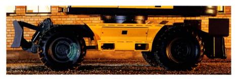
The wheel undercarriage gives you almost total freedom of choice. You can work with or without stabilizers: with four outriggers (deployed individually, simultaneously or two by two), with support blade in front and outriggers in rear, with support blades both front and rear, with only rear support blade...choose your own combination. In addition there are a number of different tyres to choose from.
