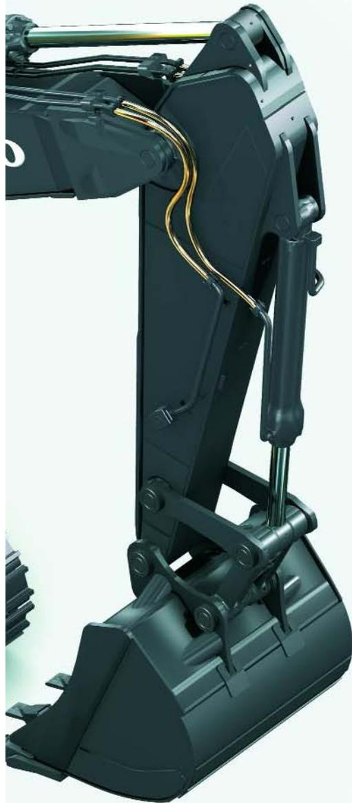
A state-of-the-art hydraulic system performs as a direct extension of the operator's thoughts and movements. That's why the B-series hydraulic system is designed with operator controllability and precision as its focus. With four different power modes, B-series hydraulics respond automatically to the operator's joystick movements and pilot pressure. This allows Volvo machines to achieve maximum efficiency on a full range of jobsites.
