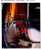
The deluxe KAB Seat (standard equipment) has 8 individual adjustments. The seat and console can be adjusted together or independently to ensure a high degree of operator comfort and to meet job site conditions.
