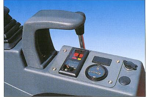
The dashboard groups together the fuel gauge, hour counter and oil pressure, water temperature and charge indicator lights. An electric socket enables an inspection lamp to be connected.
