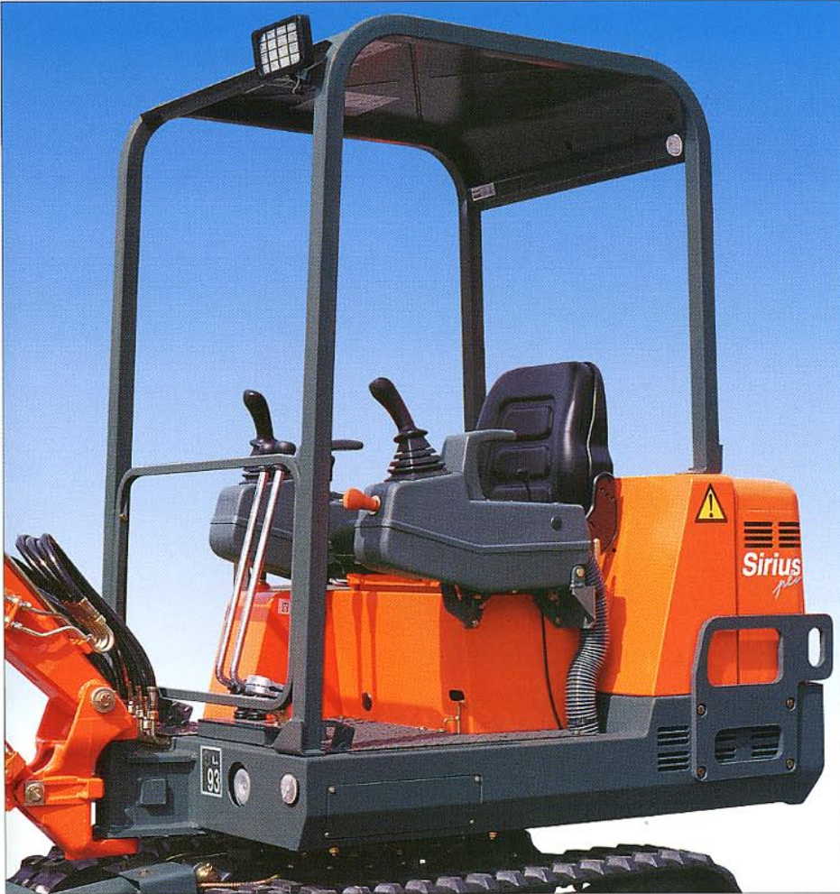
The Pel-Job canopy, which has four posts offers excellent protection. Fully glazed heated cabin is optional.
