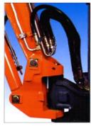
All the equipment's hoses are free and sheathed and therefore without friction or wear and are connected at the bottom of the boom for very quick replacement, if necessary. The boom is mounted on a double-swivel articulated pivot which enables a long pin to be mounted and provides greater rigidity in the boom-chassis link. The boom cylinder's rod is fully protected against any knocks by sturdy armouring.
