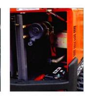
The radiators of the hydraulic circuit and engine are placed side by side to facilitate their cleaning. The battery and the air filter too are very easily accessible.
