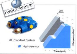
The hydrosensor valve (Pel-Job patent) on the slewing circuit damps the pressure peaks and hydraulic shocks common on starting and stopping on conventional circuits. The result: a progressive pressure increase, greater flexibility and precision and less stressed and therefore more reliable mechanical parts
