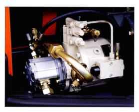
Continuous and immediate load sensing control of the hydraulic pump's flow and pressure to suit the work done by the excavator.
