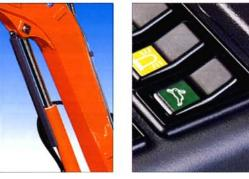
The EB 406 is provided as standard with two travel speeds, including a fast speed to speed up machine travel on the site.
