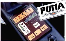
The PUMA system on the EB 406 continuously monitors all the machine's vital functions and immediately informs the operator if there is a fault. The operator is therefore free to concentrate fully on operating the machine.
