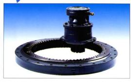
A Pel-Job exclusive: the radial piston slow slewing motor. This motor has a very high torque for flexible manoeuvres, and drives the crown directly without a mechanical reducer. The result is fewer moving parts and therefore less risk of wear. The automatic hydraulic brake integrated in the slewing motor immobilises the turret in all positions and guarantees optimum working safety even on a slope.
