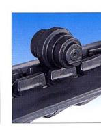
Ride comfort is considerably improved thanks to the profile of the tracks and the alternating position of the guides which provides permanent contact with the rollers.
