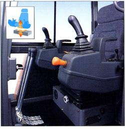
The side brackets supporting the manipulators are rigidly linked to the seat's suspension: operating precision is independent of the machine's movements and the operator is sure of finding an operating position ideally suited to him.
