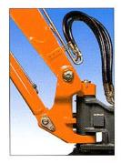
All the equipment's hoses are free and sheathed and therefore without friction or wear and are connected at the bottom of the boom for very quick replacement, if necessary. The boom is mounted on a double-swivel articulated pivot which enables a long pin to be mounted and provides greater rigidity in the boom-chassis link. The boom cylinder's rod is fully protected against any knocks by sturdy armouring.
