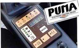
The PUMA system on the EB 30.4 continuously monitors all the machine's vital functions and immediately informs the operator if there is a fault. The operator is therefore free to concentrate fully on operating the machine.
