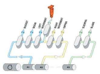
Three pumps each supply a separate hydraulic circuit in order to ensure total independence of each movement. Thus, for example, turret slewing or blade lifting are completely independent of all the equipment or travel movements.
