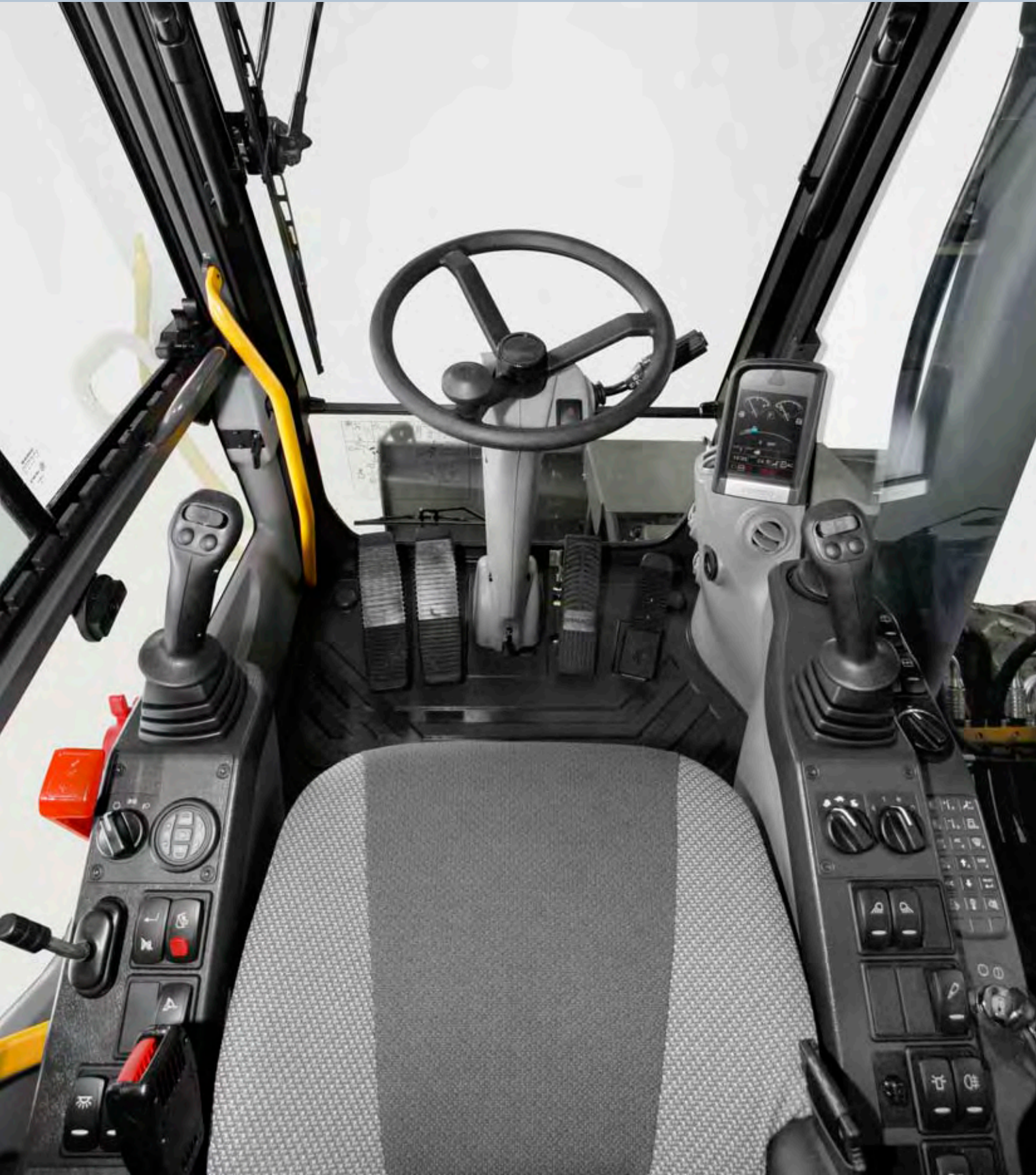
• Steering column pivots for visibility and comfort.
