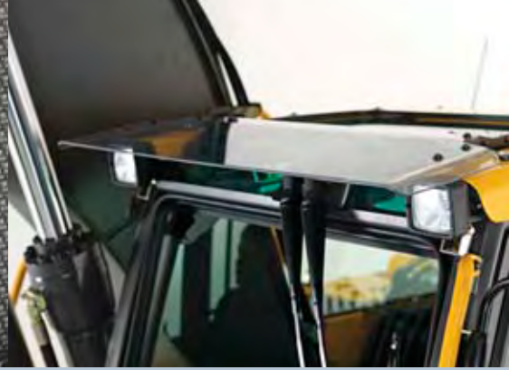
• Overhead visibility through transparent roof.
