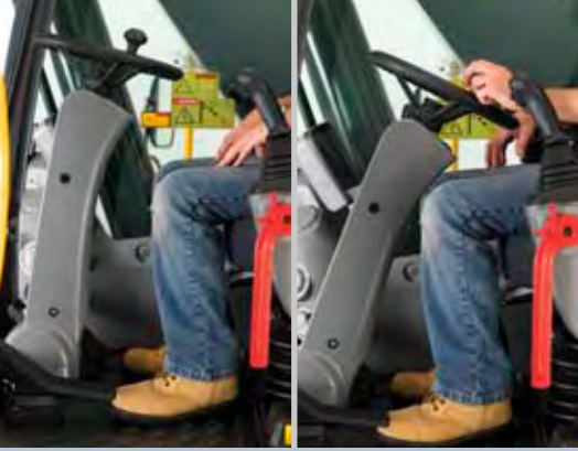
• Steering column pivots for visibility and comfort.
