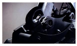
All four models, from 13 to 15 tonnes, feature hydraulic quickfit with reliable two-hand release. Unlike many others, we insist on making our own quickfits. This is the only way to guarantee the best possible match to the machine and its work duties.
