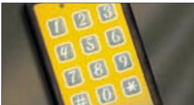
An anti-theft keypad, available as an option, enables machine starting and the main hydraulic functions to be locked.
