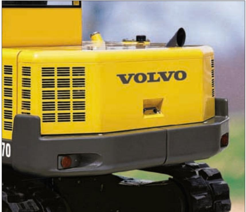
The wrap-around shape of the counterweight protects the back of the machine perfectly and makes it possible to work on the narrowest sites.
