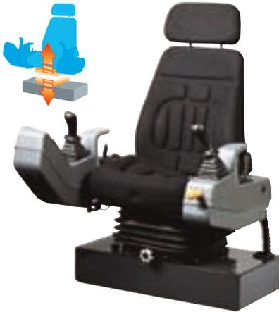
The side consoles supporting the manipulators are rigidly linked to the seat's suspension : operating precision is independent of the machine's movements and the operator is sure of finding an operating position ideally suited to him.
