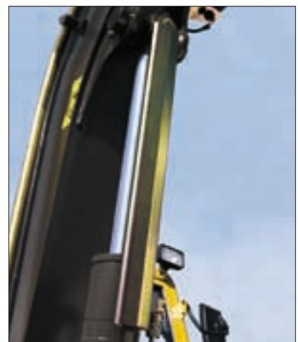
All the hydraulic hoses are sheathed and free of any friction or wear and are connected at the bottom of the boom for very quick replacement, if necessary. The boom is mounted on a double-swivel articulated pivot which enables a long pin to be mounted and provides greater rigidity in the boom-chassis link. The boom cylinder's rod is fully protected against any knocks by sturdy armoring.
