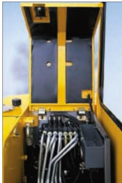
A wide central cover gives excellent access to a service platform where all the machine's hydraulic components are grouped together. Access to the control valves, rotating joint and slewing motor is immediate, which greatly facilitates all maintenance operations.
