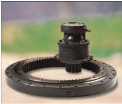
A unique feature : the radial piston slow slewing motor. This motor has a very high starting torque for flexible manoeuvres, and drives the crown directly without a mechanical reducer. The result is fewer moving parts and therefore less risk of wear. The automatic hydraulic brake integrated in the slewing motor immobilises the turret in all positions and guarantees optimum working safety even on a slope.
