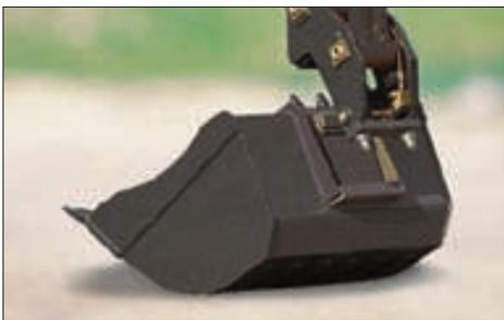
A unique feature : the quick coupling system available as an option enables bucket or accessory to be changed without the operator leaving the cab. Appreciated by all users, this device saves a lot of time and increases comfort considerably without altering the bucket's performances or sequence of operations.
