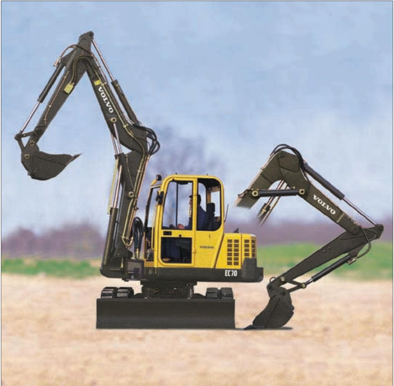
The articulated boom increases the EC70's versatility. The boom's additional joint reduces the equipment's overall dimensions and makes it possible to position the bucket on a larger ground surface, even in the immediate proximity of the machine.
