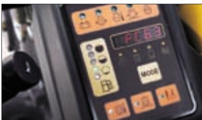
The PUMA system on the EC70 continuously monitors all the machine's vital functions and immediately informs the operator if there is a fault. The operator is therefore free to concentrate fully on operating the machine.
