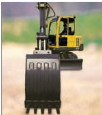
Thanks to its compact dimensions and the boom's hydraulic offset, the EC70 is at ease in all site configurations, even alongside a wall.
