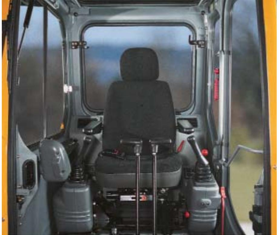
There's a single key for all locks and the ignition, and the door can even be closed from the operator's seat. The visibility is outstanding in all directions, and the wiper motor is on the cab pillar to improve visibility even further.
