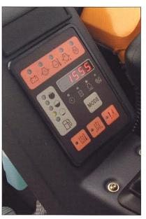
The PUMA system on the EC50 continuously monitors all the machine's vital functions and immediately informs the operator if there is a fault. The operator is therefore free to concentrate fully on operating the machine.
