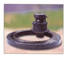
An exclusivity: the radial piston slow slewing motor. This motor has a very high starting torque for flexible manoeuvres, and drives the crown directly without a mechanical reducer. The result is fewer moving parts and therefore less risk of wear. The automatic hydraulic brake integrated in the slewing motor immobilises the turret in all positions and guarantees optimum working safety even on a slope.
