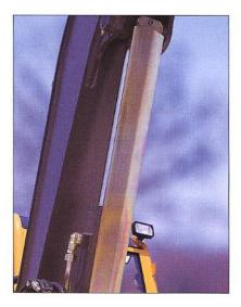
All the equipment's hoses are free and sheathed and therefore without friction or wear and are connected at the bottom of the boom for very quick replacement, if necessary. The boom is mounted on a double-swivel articulated pivot which enables a long pin to be mounted and provides greater rigidity in the boom-chassis link. The boom cylinder's rod is fully protected against any knocks by sturdy armouring.
