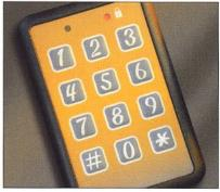
An anti-theft keypad, available as an option, enables machine starting and the main hydraulic functions to be locked
