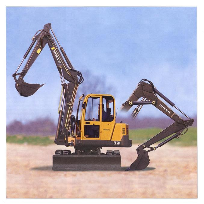
The articulated boom increases the EC50's versatility. The boom's additional joint reduces the equipment's overall dimensions and makes it possible to position the bucket on a larger ground surface, even in the immediate proximity of the machine.
