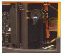
The radiators of the hydraulic circuit and engine are placed side by side to facilitate their cleaning. The battery and the air filter too are very easily accessible.
